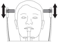
Carefully press the head supports by hand towards the head in order to check that they are in the right position. The device or the head supports are not damaged in the process. Ideally, the head supports should make contact slightly above the eye brows; correct the position as required. Close the head supports with the button. To do this, just press the button briefly – don't press and hold.
