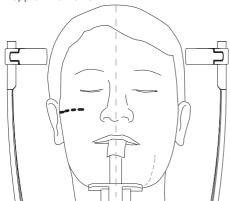
Fig. 3: Frankfurt plane: laser height to the lower edge of the eyes
