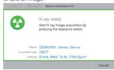
Trigger the image by pressing and holding the button on the exposure switch until the acoustic signal stops and the control lamp goes out. The scan times depend on the patient type, imaging program and image quality (see "12 Program parameters").
