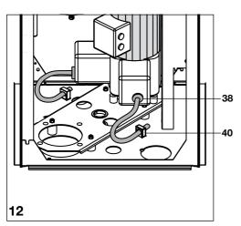
Place the noise reducers (38) onto the suction connections of the unit and fix in place using the securing clamps (40).
